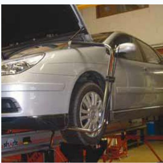
Measuring of high test point (Mc Pherson)
