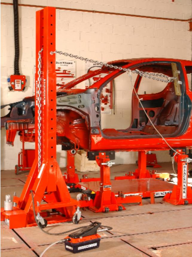
For users of the Korek® frames wishing to have a mobile pulling device, complete and ready-to-use. The 10-tonne pulling force allows working on small commercial vehicles. With its vertical extensions, pull 2.80 metres from the ground with a force of 2 tons.
